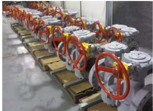
Interlock systems for valve manifolds
