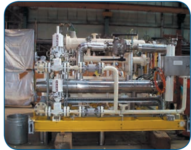
The valves illustrated are 4" class 300 flanged in Carbon Steel and Stainless Steel. The application is on a fuel skid and both plugs on each valve are lever operated. Criteria for selection: double block and bleed with true bubble tight isolation for reasons of safety, reliability and minimum maintenance.
